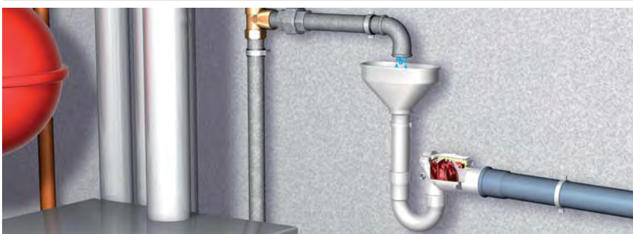
... furnace condensation overflow
